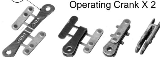
Hand Brake Operating Crank X 2
