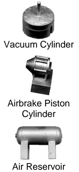
When vans were modified to dual air and vacuum brakes. The inboard vee hangers were moved to the outer Solebars and longer cross shafts fitted. One vacuum cylinder was moved to sit alongside The other (against the air piped solebar). Airbrake piston cylinder and a air reservoir cylinder were fitted into the vacated space (on the vacuum piped solebar side). Cranks and linkage were fitted so that the two cross shafts would rotate together when the air brake piston operated.
